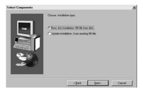
Choose **NEW**, **FIRST INSTALLATION** if you want to install *BoardMaster* and your Circuit Board Plotter the first time on this computer. The setup program will ask you to insert the configuration disk into drive A:, which has been delivered with your Circuit Board Plotter and contains the individual INI-file. If you <u>don't</u> want to use your configuration disk to install *BoardMaster* with default parameters, press **<ESC>**.
